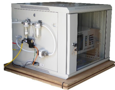
Siloxane Monitor housed in 19" rack cabinet
